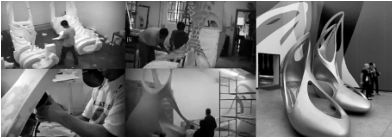
Fig.5 Handcraft fabrication process of a digital designed complex geometry shape. Fiberglass finished on top of foam block and wooden ribs structure.
